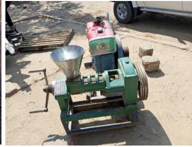
Oil expeller not installed
