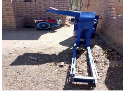
Hammer mill not installed
