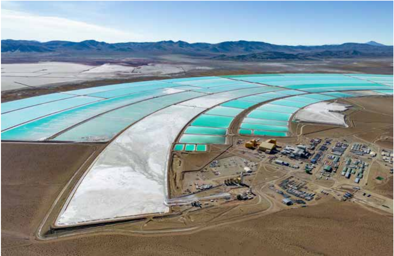
Photo: Aerial view of lithium fields or evaporation ponds in the highlands of northern Argentina. Credit: Freedom_wanted, Shutterstock.
