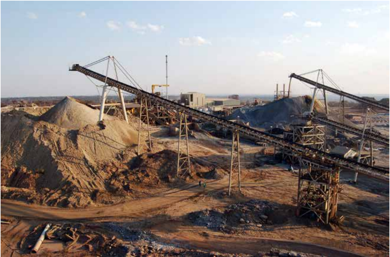
Photo: Conveyor belts feed broken rock into two different stockpiles (oxides and sulphides) at an open-pit copper mine in Zambia. Credit: Africanway, iStock.
